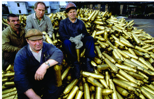
Figure 1: Thousands of brass shells in Russian military storage were melted-down for use in the CMS detector (from [3])
